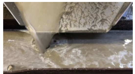
Up to 80 liters of water per cubic meter are drained during the pressing process © Saalasti
