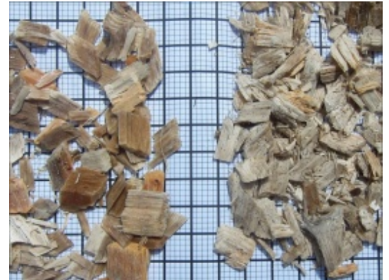
The structure of the wood is broken up during the pressing process which improves the pellets' color, homogeneity and strength © Saalasti
