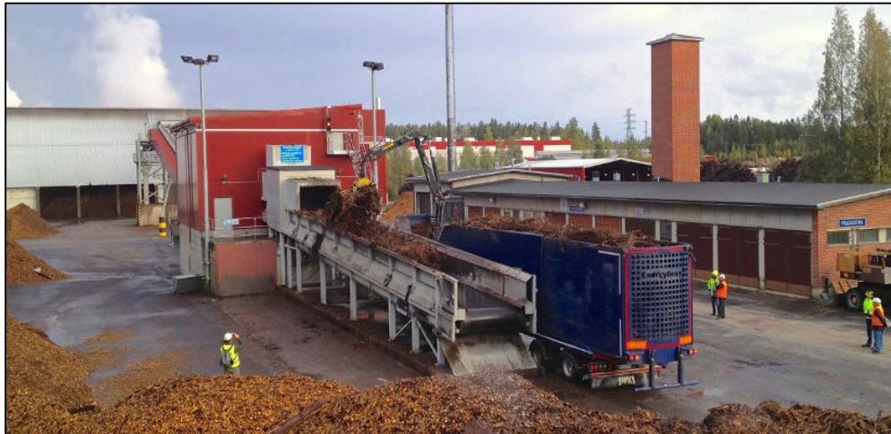
Saalasti Crush 1224H installation processing stumps in Kaipola, Finland
