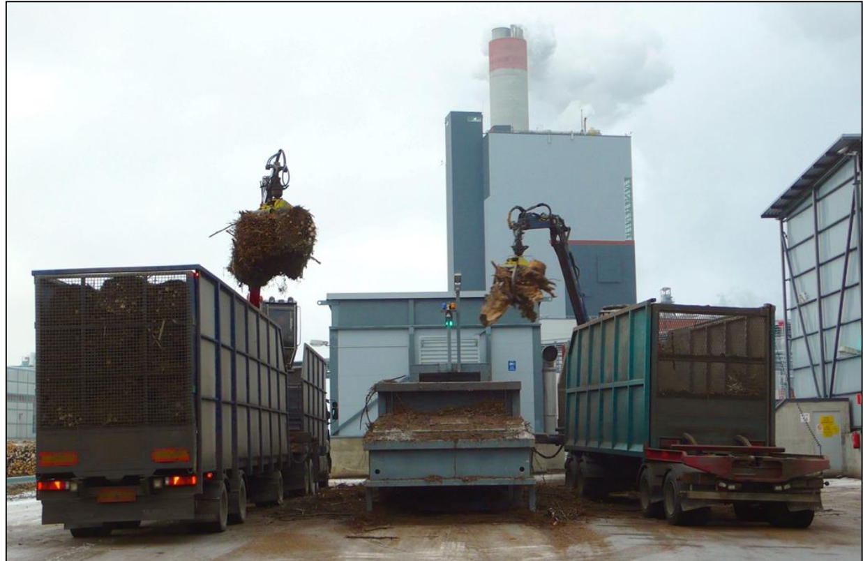
Saalasti Crush 1224H processing stumps and forest residue bundles in Kyminvoima Finland
