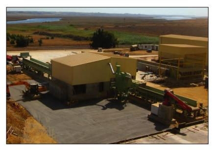
Saalasti Crush 1224H processing euca stumps in Spain Huelva (Ence)
