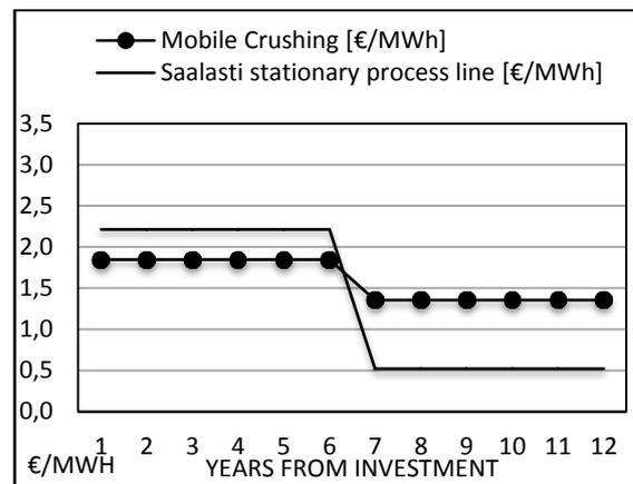
**Figure 8:** The crushing cost over time with the electric powered mobile crusher and Saalasti's stationary crusher process line, case two with reduced annual production of the stationary crushing line.
