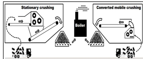
**Figure 2:** The flow sheets of the case two's crushing processor options compared in the cost analysis
