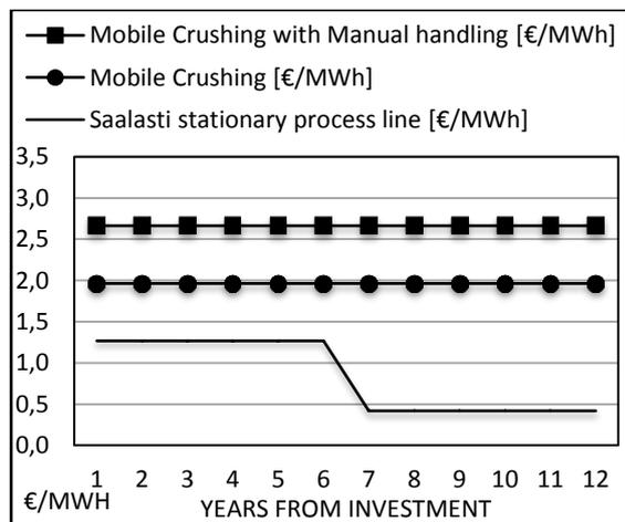
**Figure 4:** The crushing cost over time with the diesel powered mobile crusher and Saalasti's stationary crusher process line, case one.
